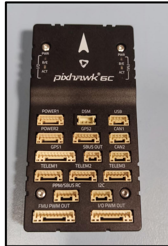
Figure 3.19: Pixhawk 6C Controller
