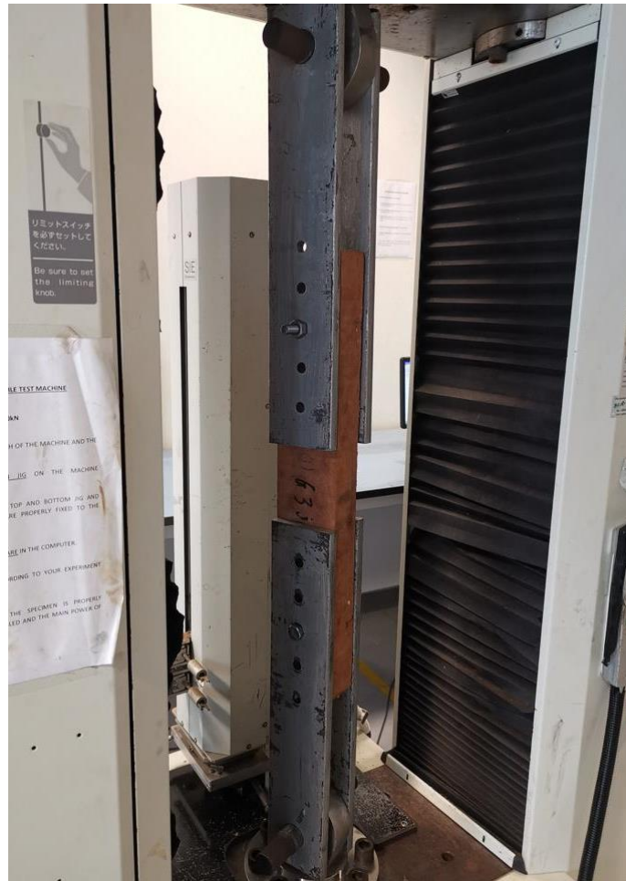
Figure 3.8: Test Set-Up of Timber Bolted Connection Testing
