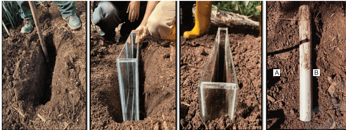
Figure 3. The scanner box installation. The soil was dug and the scanner box was inserted vertically. A half-open PVC pipe was then placed to cover the scanner box. 'A' side is facing the palm and 'B' side is away from the palm.
