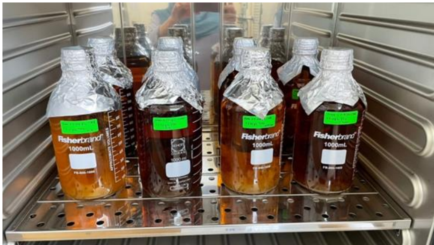
Figure 3.13: Accelerated thermal ageing experiment using a convection oven
