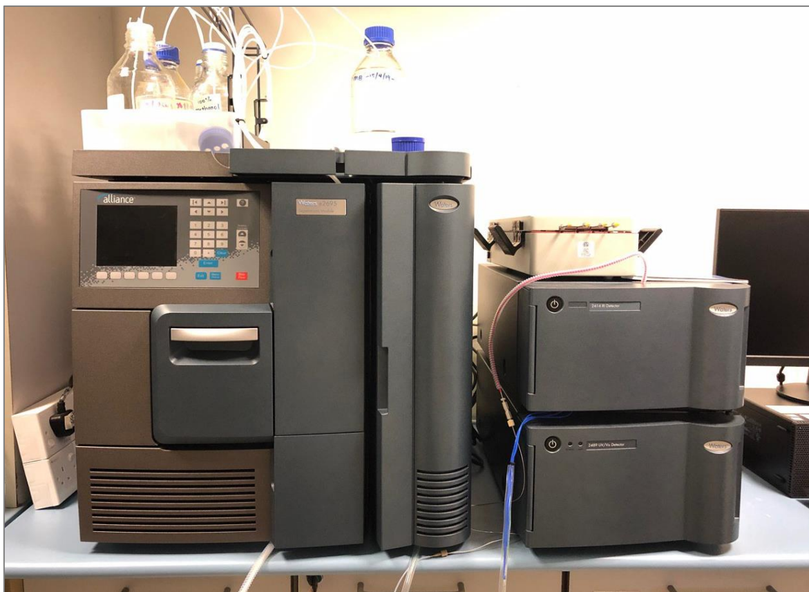
Figure 3.13: Main components of High-Performance Liquid Chromatography (HPLC), which consists of a pump, injector, column, detector and integrator and display system.
