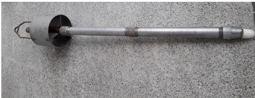
Figure 3.3: Gravity corer for core sediments collection
