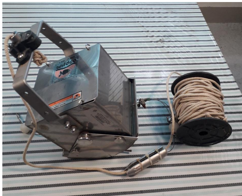
Figure 3.2: Grab sampler for surface sediment collection
