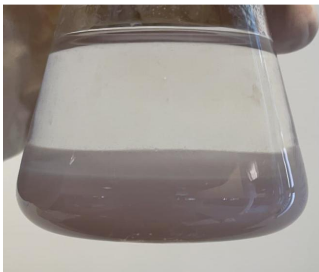
Figure 3.1: Purple colloid formed after hydrothermal treatment at 70 \pm 2 °C
