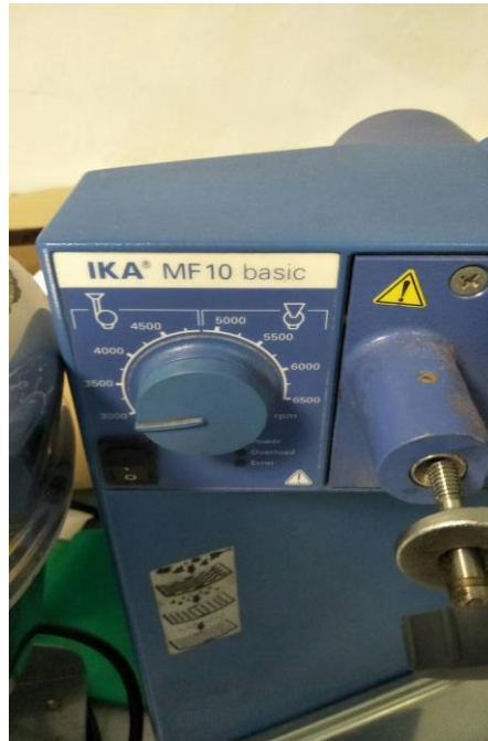
Figure 3.3: IKA® MF10 basic to grind sago log into sawdust
