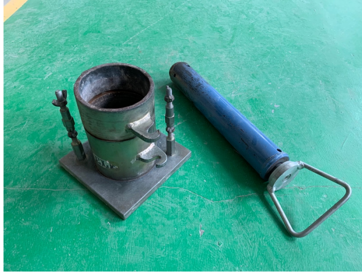
Figure 3.6: Mould and Proctor Hammer used in the Standard Compaction Test.
