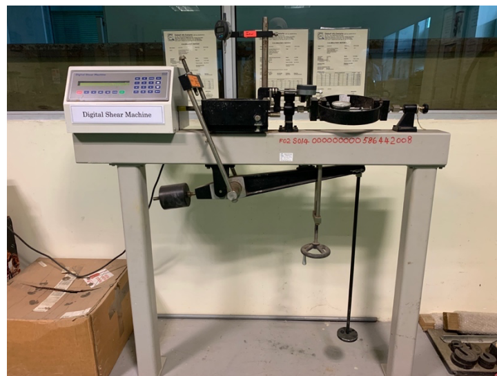
Figure 3.7: Direct Shear Box
