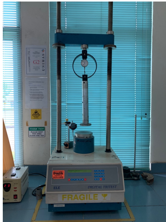
Figure 3.8: Experimental set up of unconfined compression test
