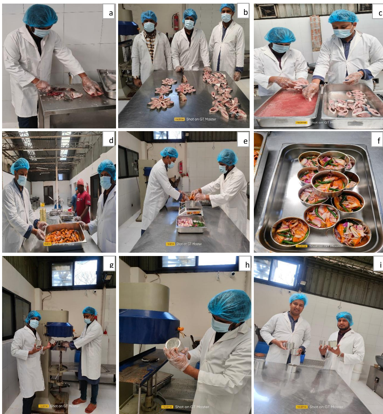
Figure 5.2: Different steps of processing of canned hilsa; a) dressing of fish, b) dressed hilsa, c) washing, d) marinating, e) weighing, f) Can filling, g) Sealing of can, h) checking double seaming, i) processed canned hilsa.
