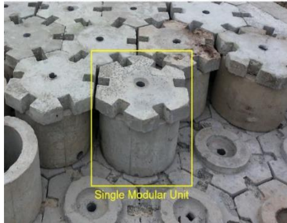
Figure 2.16: Single Modular Unit of StormPav (Mah et al., 2018b)
