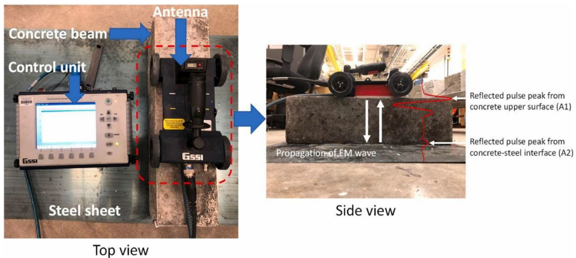
Fig. 5 Use of ground penetrating radar on concrete sample [8]
