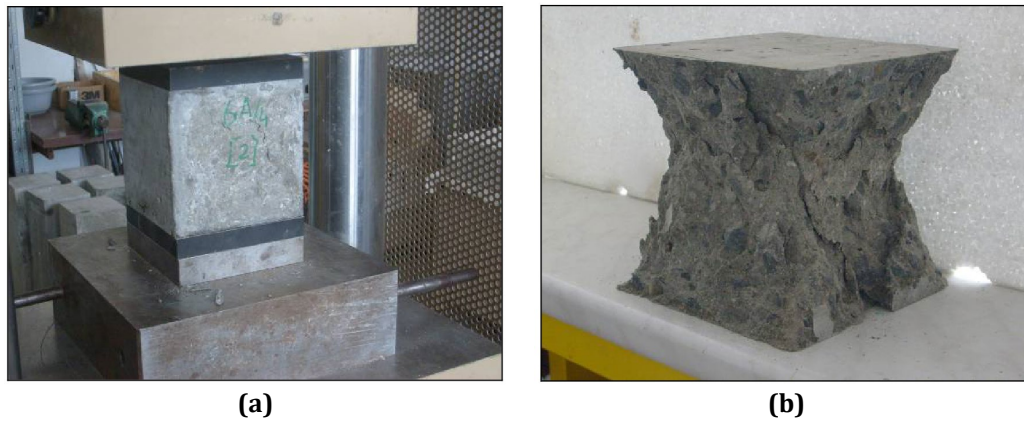
Fig. 1 Strength testing on concrete (a) Under compressive test machine; (b) Cube sample after testing [1]
