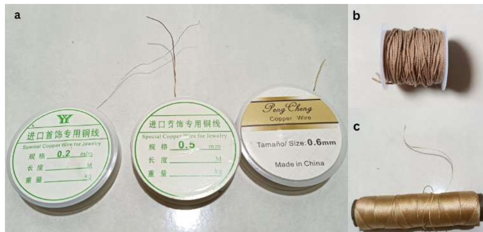
Figure 4.17: a) Copper wires, b) cotton thread, and c) nylon twine
