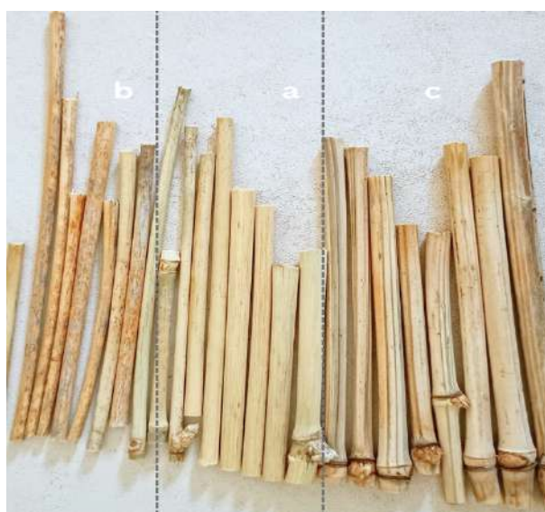
Figure 4.6: Three types of bamboo branches boiled with alum
