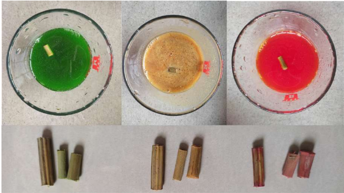
Bamboo in a limestone solution with food colorings
