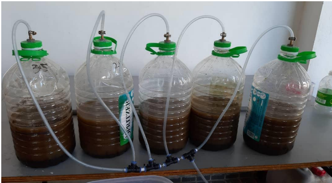
Figure 3.3: Experimental Set-up of 5L Reactor
