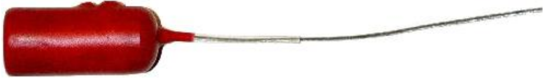
Figure 4.2: Holohil SB-2 (Holohil Systems Ltd, Canada) radio transmitter used for female Tropidolaemus subannulatus .
