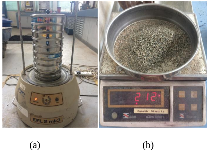
Figure 3.12: (a) Sieve analysis of samples (b) weighted sample retained in sieve
