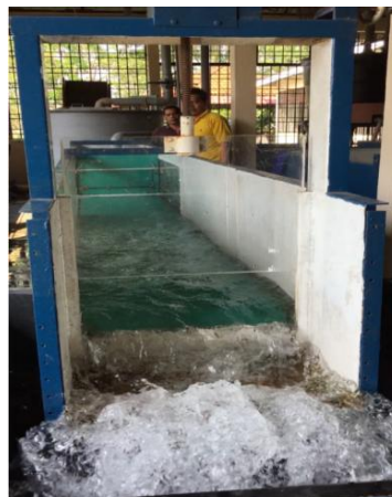
Figure 3.6: Flush gate operation experiment
