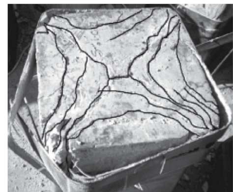
Fig. 1 Concrete confinement mechanisms: a Comparative confinement behavior across section geometries (Li et al., 2025; b Typical cracking pattern in confined square concrete section (Youssef et al., 2007)
