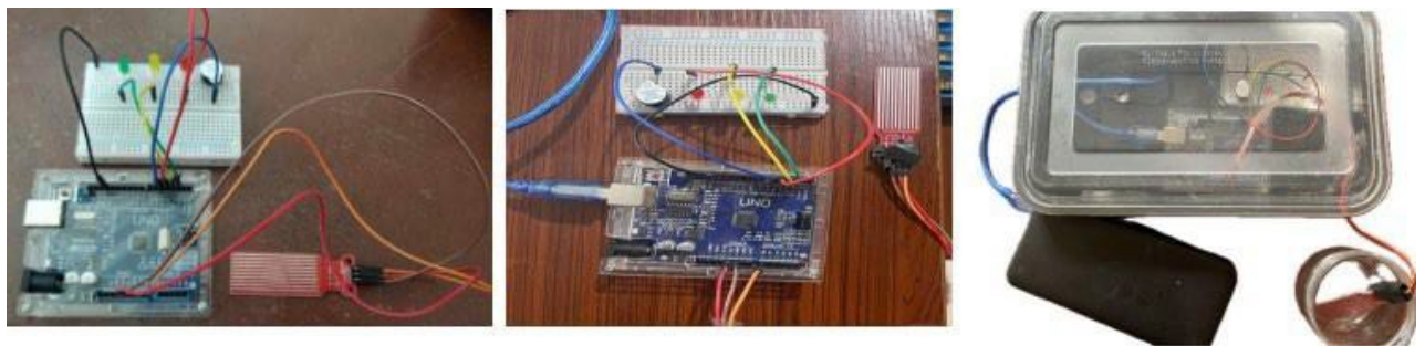
Figure 2.4: Actual Product of Automated flood water level sensor and alarm system using Arduino Uno (Magnaye et al., 2024)
