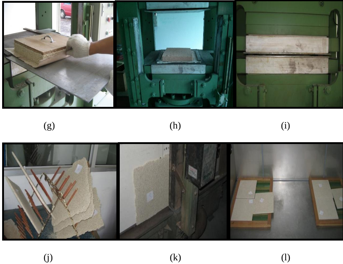
Figure 3.1: Sago composite particleboard production process (a) Mixing preparation of sago particles (b) Mixing process of sago and with (c) Adhesive spraying process (d) The mixture of sago composite (e) Mixture was manually compressed (f) Steel bars with 10mm thickness for setting (g) Transferring the mixture from mold (h) Sago composite mixture for hot press process (i) Mixture being compressed as sago composite particleboard (j) Heat released after the fabrication (k) Cutting process for sago composite particleboard (l) Curing process for sago composite particleboard.
