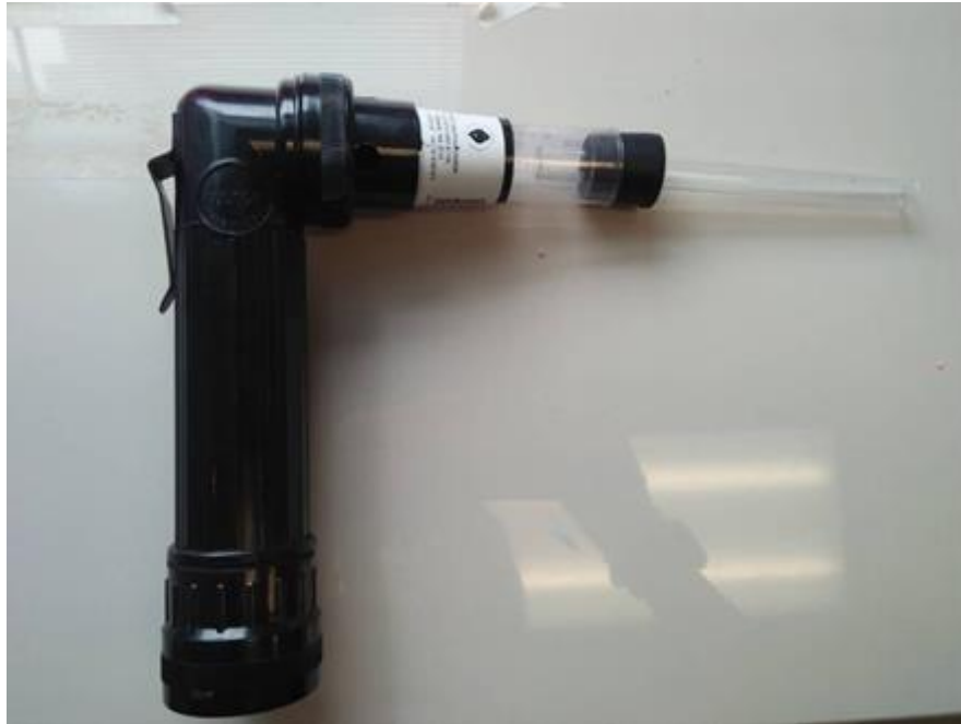
Appendix FIII: Mechanical aspirator used to collect adult mosquitoes from the field
