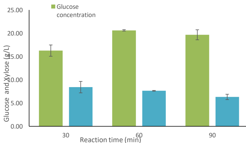
Figure 4.2: Effects of different reaction time on xylose and glucose concentration during high pressure steam autoclave pre-treatment. Error bars indicate the mean \pm standard deviation of duplicate experiments.
